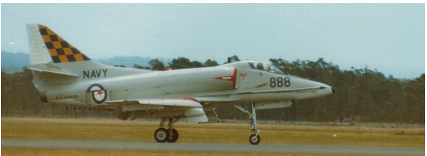
A-4G "888" served primarily all of its life with VF805, though briefly in the mid seventies, it did serve with VC724. Note replacement offset bent shorter refuelling probe now installed.
