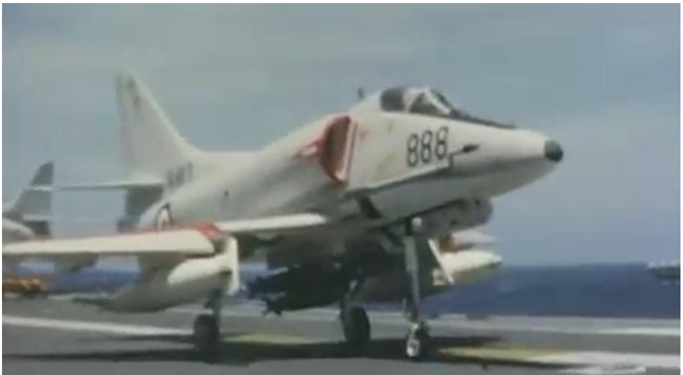
"888" loaded with two tanks and three bombs on a central triple carriage.
