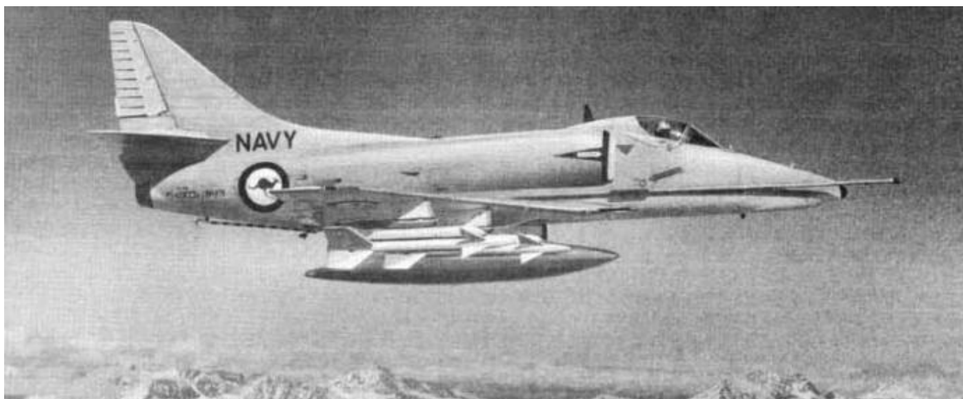
High over the US of A, our first A-4G N13-154903 carries the RANFAA standard four sidewinder load.
