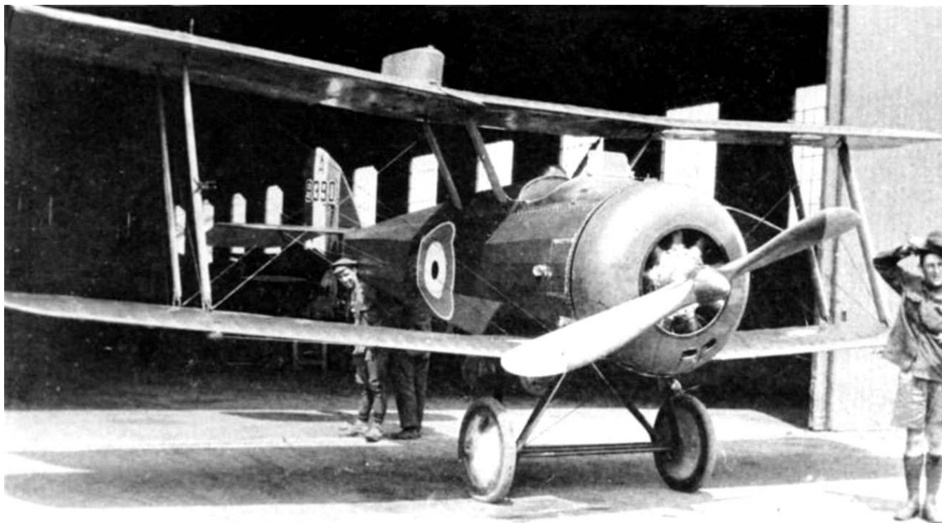
A9390 in AUG 1917 at Harlaxton – this is before modification with the six cowl stiffening ribs added to reduce vibration of the Le Rhône rotary engine, which regularly shed its valve tappet rods [AWM P004522]
