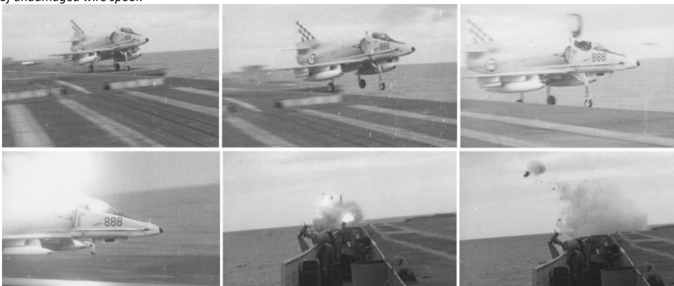
Then in sequence; cable lets go, spools off, but still causes drag on arrestor hook, "888" just has no adequate air speed to initiate an aborted go around. As it nears the edge of the flight deck, the pilot is already initiating his ejection seat escape. Canopy blows, and with sink rate increasing as it clears the deck, he is successfully ejected. It became RAN Ejection number 9.
