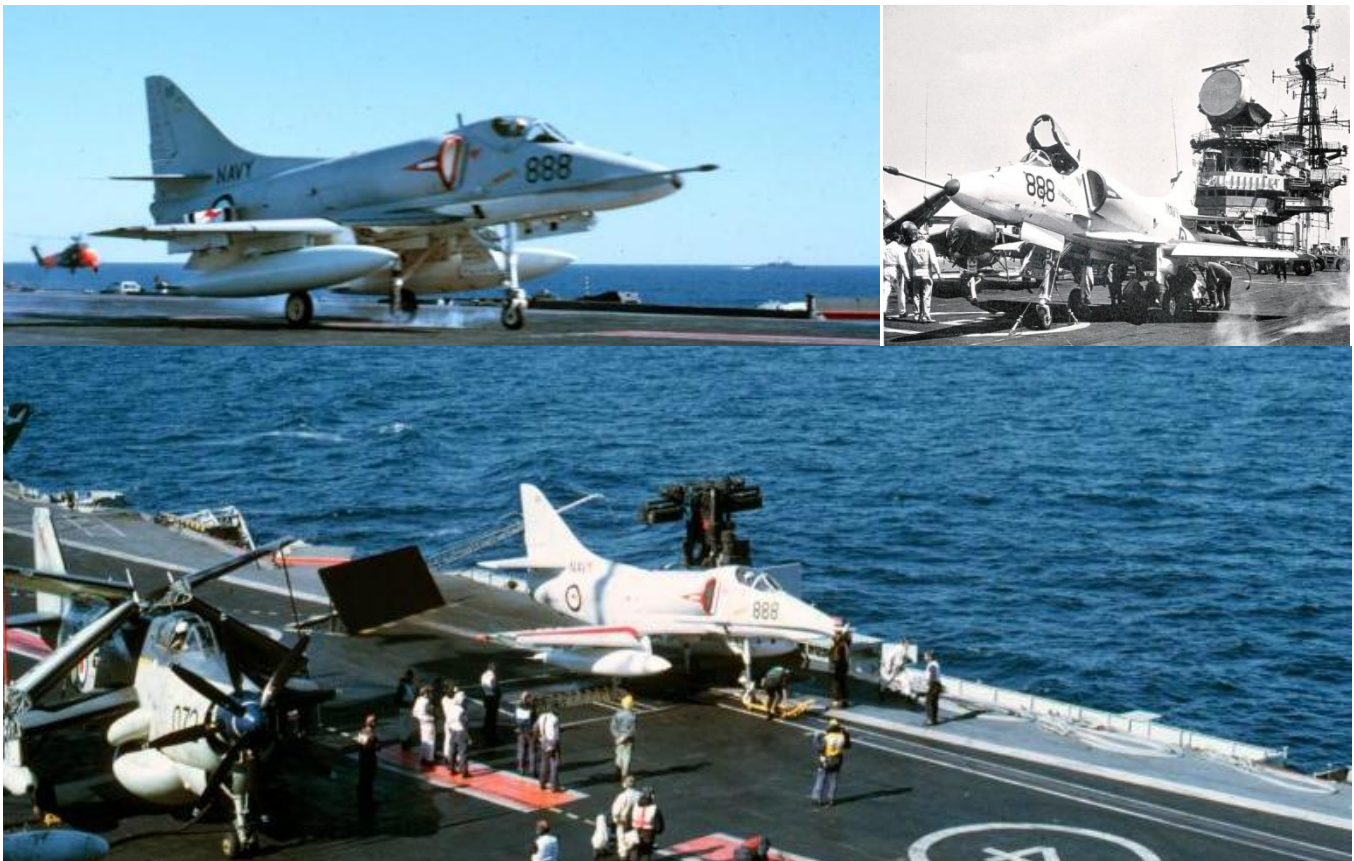
A-4G "888" pictured after landing and later catapulting of HMS Hermes and note, the original straight offset refuelling probe. Fourteen years later, in the South Atlantic, the very type would be deemed as the enemy to HMS Hermes.
